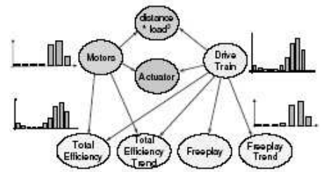
Fig. 7. Bayesian Network Model for Flight Actuator - Structure and Distributions. Motors and Drive Train represent components, Actuator is a subsystem, the node at the top stands for evidence of usage and the four nodes along the bottom represent present and future health evidence.
